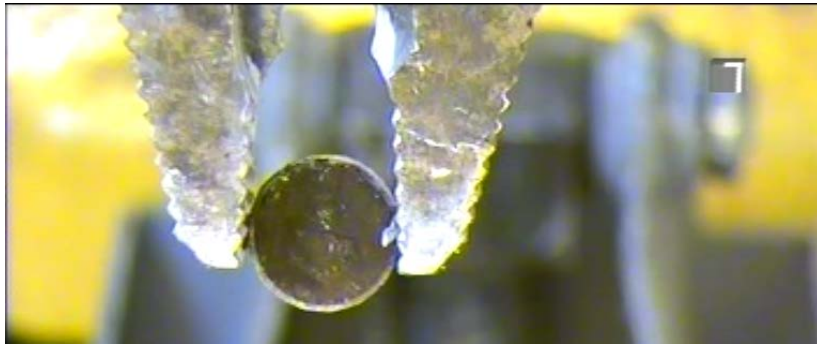
Figure 7 - Small item held in HCS7 shear paddles (CCTV still)
